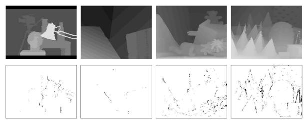
Figure 3: Propagation process results for the four Middlebury stereo pairs (Tsukuba, Venus, Teddy, Cones). From the top to the bottom: The produced disparity maps, disparity errors (marked in black) in all regions with 1 pixel error threshold.
