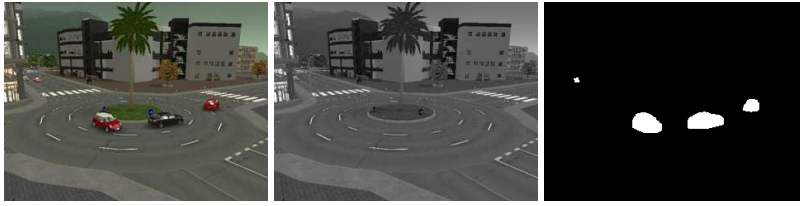
Fig. 1 Background Modeling and Foreground Detection: Original image (309), reconstructed background image, foreground mask (Sequences from BMC 2012 dataset [552]).
