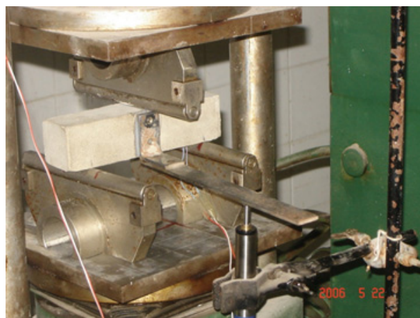
FIGURE 3. Three point bending test setup.
