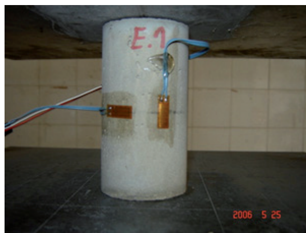
FIGURE 4. Test setup of the cylinder GFRC.
