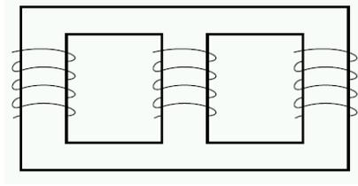
Figure 2. Magnetic circuit
