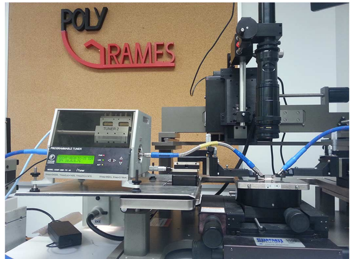
Fig. 8. Picture of part of the setup used to compare the PCE of the HSMS-2850 and backward tunnel diode. The picture shows the probe station and the Focus Microwaves Tuner, used as matching network.
