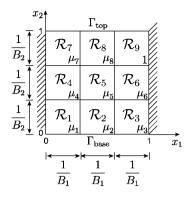
**Fig. 11** Thermal Block problem for  $B_1 = B_2 = 3$
