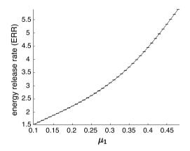
**Fig. 28** Elastic Crack problem:  $\widehat{G}_N^{\mathcal{N}}(\boldsymbol{\mu})$  and the error bar interval  $[\widehat{G}_N^{\mathcal{N}}(\boldsymbol{\mu}) - \Delta_N^{\widehat{G}}(\boldsymbol{\mu}), \widehat{G}_N^{\mathcal{N}}(\boldsymbol{\mu}) + \Delta_N^{\widehat{G}}(\boldsymbol{\mu})]$  for  $\mu_1 \in [0.1, 0.45], \mu_2 = 0.25$ , and N = 30
