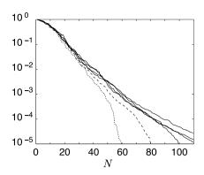
Fig. 24 Thermal Block problem for  $B_1 = B_2 = 3$ : (upper bound for the)  $L^{\infty}(\Xi_{\text{train}})$  relative energy error, (82), as a function of N;  $\mathcal{N} = 137$  (*dotted*),  $\mathcal{N} = 453$  (*dashed*), and  $\mathcal{N} = 661$ , 1737, 2545, 6808 (all quite similar)
