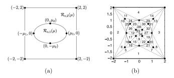
**Fig. 9** (a) Original domain  $\Omega_0(\mu)$  with  $L_{\text{reg}} = 2$  regions  $\mathcal{R}_{0,1}(\mu)$  and  $\mathcal{R}_{0,2}(\mu)$  and initial control points/edges indicated, and (b)  $K_{\text{dom}} = 34$  RB triangulation  $\overline{\Omega} = \bigcup_{k=1}^{K_{\text{dom}}} \overline{\Omega}^k$
