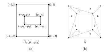
**Fig.** 7 (a) Original domain  $\Omega_0(\mu)$  with single region  $\mathcal{R}_{0,1}(\mu)$  and initial control points/edges indicated, and (b)  $K_{\text{dom}} = 8$  RB triangulation  $\overline{\Omega} = \bigcup_{k=1}^{K_{\text{dom}}} \overline{\Omega}^k$  (the numbers refer to subdomains)
