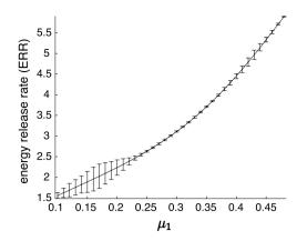
**Fig. 27** Elastic Crack problem:  $\widehat{G}_N^{\mathcal{N}}(\boldsymbol{\mu})$  and the error bar interval  $[\widehat{G}_N^{\mathcal{N}}(\boldsymbol{\mu}) - \Delta_N^{\widehat{G}}(\boldsymbol{\mu}), \widehat{G}_N^{\mathcal{N}}(\boldsymbol{\mu}) + \Delta_N^{\widehat{G}}(\boldsymbol{\mu})]$  for  $\mu_1 \in [0.1, 0.45], \mu_2 = 0.25$ , and N = 15
