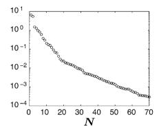
**Fig. 26** Inviscid flow example:  $\max_{\mu \in \Xi} \operatorname{train} (\Delta_N^{\mathrm{en}}(\mu)/|||u_N^N(\mu)|||_{\mu})$  as a function of *N* for the Lagrange RB approximations associated with the sample of Fig. 25; here  $\Xi_{\mathrm{train}}$  is a log-uniform random sample of size  $n_{\mathrm{train}} = 3000$
