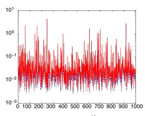
**Fig. 31** Advection-Diffusion problem:  $\alpha_{\text{UB}}^{\mathcal{N}}(\mu)$  (*upper curve, solid*) and  $\alpha_{\text{LB}}^{\mathcal{N}}(\mu)$  (*lower curve, dotted*) as a function of  $\mu' \in \Xi_{\text{train,SCM}}$  after  $J_{\text{max}} = 4$  iterations of the SCM greedy algorithm; here the abscissare represents the index of the point  $\mu_{\text{train,SCM}}^k$  in  $\Xi_{\text{train,SCM}}$
