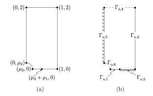
**Fig. 14** Elastic Crack: (a) Original domain  $\Omega_0(\mu)$  (single region) with initial control points/edges indicated, and (b) Boundary segments on  $\partial \Omega_0(\mu)$
