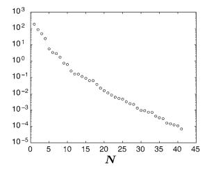
**Fig. 30** Advection-Diffusion problem:  $\max_{\mu \in \Xi_{\text{train}}} \Delta_N^s(\mu)$  as a function of *N*; note  $|s^{\mathcal{N}}(\mu) - s_N^{\mathcal{N}}(\mu)| \le \Delta_N^s(\mu)$
