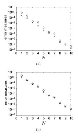
**Fig. 20** Thermal Block problem for  $B_1 = 2$ ,  $B_2 = 1$ : (a)  $\|u^{\mathcal{N}} - u_N^{\mathcal{N}\text{POD}}\|_{L^2(\Xi;X)}$  (×) and  $\|u^{\mathcal{N}} - u_N^{\mathcal{N}\text{Greedy}}\|_{L^2(\Xi;X)}$ ( $\diamond$ ) as a function of N; (b)  $\|u^{\mathcal{N}} - u_N^{\mathcal{N}\text{POD}}\|_{L^{\infty}(\Xi;X)}$  ( $\diamond$ ) and  $\|u^{\mathcal{N}} - u_N^{\mathcal{N}\text{Greedy}}\|_{L^{\infty}(\Xi;X)}$  ( $\diamond$ ) as a function of N
