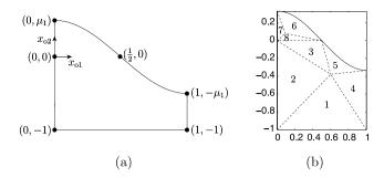
**Fig. 10** (a) Original domain  $\Omega_{\rm o}(\mu)$  with single region  $\mathcal{R}_{\rm o,1}(\mu)$  and initial control points/edges indicated, and (b)  $K_{\rm dom} = 8$  RB triangulation  $\overline{\Omega} = \bigcup_{k=1}^{K_{\rm dom}} \overline{\Omega}^k$
