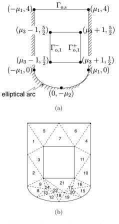
**Fig. 12** (a) Original domain  $\Omega_0(\mu)$  with single region  $\mathcal{R}_{0,1}(\mu)$  and initial control points/edges indicated, and (b)  $K_{\text{dom}} = 22 \text{ RB}$  triangulation  $\overline{\Omega} = \bigcup_{k=1}^{K_{\text{dom}}} \overline{\Omega}^k$
