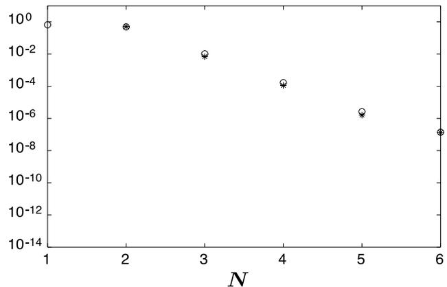
**Fig. 18** Thermal Block problem for  $B_1 = 2$ ,  $B_2 = 1$ :  $L^\infty(\mathcal{E})$  relative energy error as a function of  $N$  for the spaces  $W_N^{\mathcal{N}\text{nh,ln}}$  (\*) and  $W_N^{\mathcal{N}\text{Greedy,en}}$  (o) ((78) and (79), respectively)
