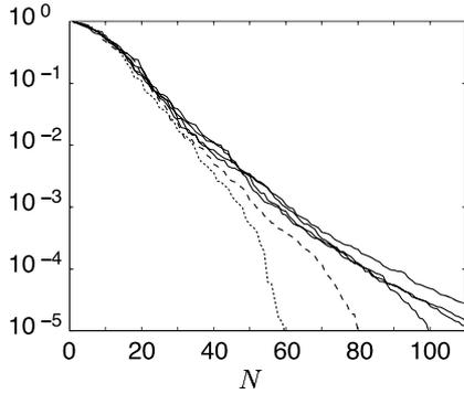
**Fig. 24** Thermal Block problem for  $B_1 = B_2 = 3$ : (upper bound for the)  $L^\infty(\mathcal{E}_{\text{train}})$  relative energy error, (82), as a function of  $N$ ;  $\mathcal{N} = 137$  (dotted),  $\mathcal{N} = 453$  (dashed), and  $\mathcal{N} = 661, 1737, 2545, 6808$  (all quite similar)
