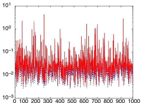
**Fig. 31** Advection-Diffusion problem:  $\alpha_{\text{UB}}^N(\boldsymbol{\mu})$  (upper curve, solid) and  $\alpha_{\text{LB}}^N(\boldsymbol{\mu})$  (lower curve, dotted) as a function of  $\boldsymbol{\mu}^k \in \mathcal{E}_{\text{train,SCM}}$  after  $J_{\text{max}} = 4$  iterations of the SCM greedy algorithm; here the abscissa represents the index of the point  $\boldsymbol{\mu}_{\text{train,SCM}}^k$  in  $\mathcal{E}_{\text{train,SCM}}$
