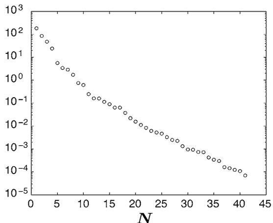
**Fig. 30** Advection-Diffusion problem:  $\max_{\boldsymbol{\mu} \in \mathcal{E}_{\text{train}}} \Delta_N^s(\boldsymbol{\mu})$  as a function of  $N$ ; note  $|s^N(\boldsymbol{\mu}) - s_N^N(\boldsymbol{\mu})| \leq \Delta_N^s(\boldsymbol{\mu})$
