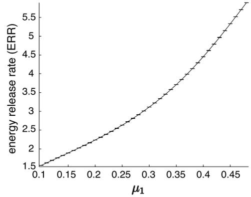
**Fig. 28** Elastic Crack problem:  $\widehat{G}_N^{\mathcal{N}}(\boldsymbol{\mu})$  and the error bar interval  $[\widehat{G}_N^{\mathcal{N}}(\boldsymbol{\mu}) - \Delta_{\widehat{G}_N^{\mathcal{N}}}(\boldsymbol{\mu}), \widehat{G}_N^{\mathcal{N}}(\boldsymbol{\mu}) + \Delta_{\widehat{G}_N^{\mathcal{N}}}(\boldsymbol{\mu})]$  for  $\mu_1 \in [0.1, 0.45]$ ,  $\mu_2 = 0.25$ , and  $N = 30$
