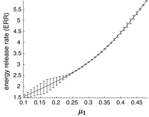
**Fig. 27** Elastic Crack problem:  $\widehat{G}_N^{\mathcal{N}}(\boldsymbol{\mu})$  and the error bar interval  $[\widehat{G}_N^{\mathcal{N}}(\boldsymbol{\mu}) - \Delta_{\widehat{G}_N^{\mathcal{N}}}(\boldsymbol{\mu}), \widehat{G}_N^{\mathcal{N}}(\boldsymbol{\mu}) + \Delta_{\widehat{G}_N^{\mathcal{N}}}(\boldsymbol{\mu})]$  for  $\mu_1 \in [0.1, 0.45]$ ,  $\mu_2 = 0.25$ , and  $N = 15$
