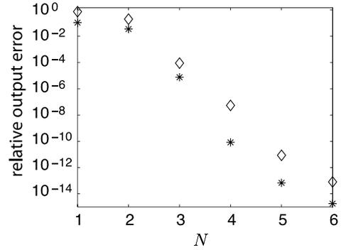
**Fig. 21** Thermal Block problem for  $B_1 = 2$ ,  $B_2 = 1$ : Relative output error as a function of  $N$  for the output interpolant (\*) and RB output prediction ( $\diamond$ ) ((80) and (81), respectively)
