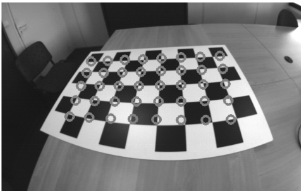
Fig. 3: Initial approximation of the transformation between the board and the camera — the reprojected grid is represented by gray circles.
