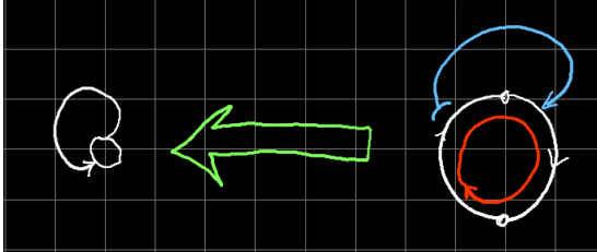
Figure 3.13: A 0 length path (an example of 0 length path is the self-inductance of a loop)
