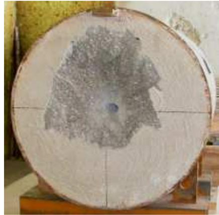
Fig. 5 : Penetration depth versus initial kinetic energy and front face of target after shot ( $V_i=227$  m/s)
