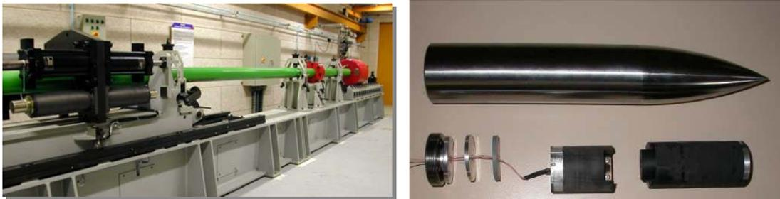
Fig. 4 : Gas launcher and rigid projectile with its acceleration recorder system
