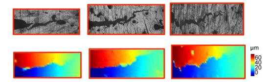
Fig. 3 – Vertical displacement field calculated by Digital Image cross-Correlation as the main cracks grow in the 3 bone samples where the osteons are either in the longitudinal, anti-plane longitudinal or transverse directions respectively.
