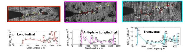
Fig. 6 – Stress intensity factors calculated by total energy variation in the three bone characteristic directions: longitudinal, anti-plane longitudinal, transverse.
