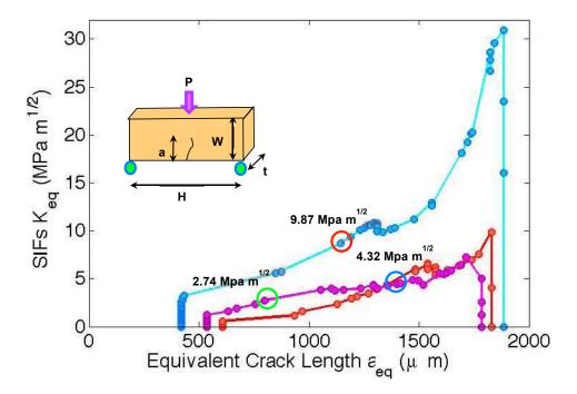
Fig. 5 – The stress intensity factors are calculated following ASTM Standard E399 which uses a analytical formula for homogeneous materials.
