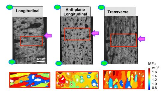
Fig. 2 – Young's moduli map in the windows of observation in the vicinity of the crack indent of the 3 bone samples where the osteons are either in the longitudinal, anti-plane longitudinal or transverse directions respectively.
