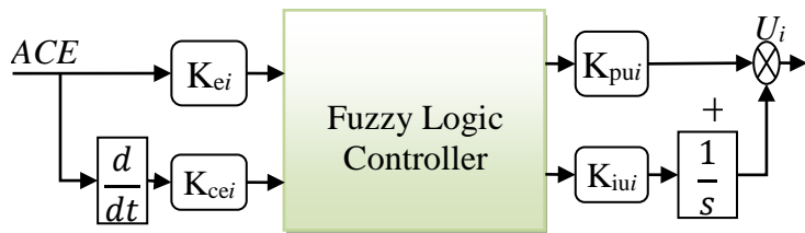
Figure 4. Fuzzy Logic Controller for i-Area, where i=1 & 2
