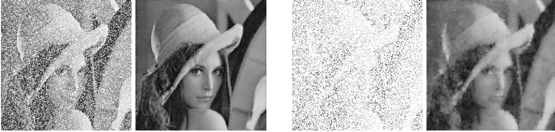
FIGURE 11. Two inpainting via the DR method of images missing, respectively, 30% and 80% of pixels. For both images we chose T = 1 and n = 60 steps. Notice how in the second image, the big corruption makes it difficult to correctly compute the gradient.
