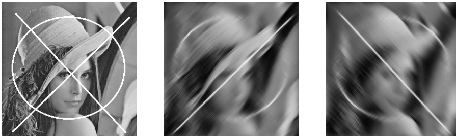
FIGURE 8. Hypoelliptic diffusion of lift with fixed angle \theta_0 . Left: original image. Middle: \theta_0 = \frac{\pi}{4} . Right: \theta_0 = \frac{3\pi}{4} . In particular observe that only the white stripe perpendicular to \theta_0 is filled, while the other is preserved.
