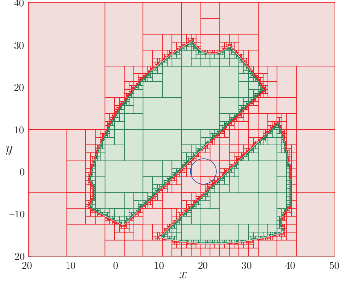
Fig. 5. The obstacle-free workspace, considering only edge B_1 B_2 of EE, for \phi = \pi/4 . This is a modified result of Fig. 4. A better solution is represented in Fig. 7(a).
