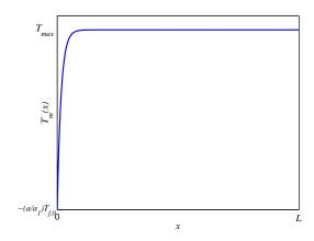
**Figure 2.** Temperature distribution in the metallic tube  $T_m$
