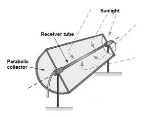
Figure 1. Cylindro-parabolic solar collector [2]
