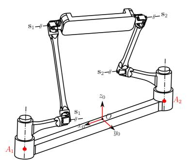
Figure 3: A pose in the third mode  $\mathcal{K}_3$ .
