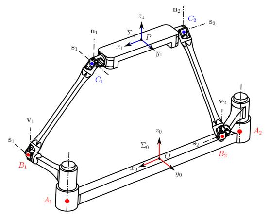
Figure 1: The 2-RUU parallel manipulator.
