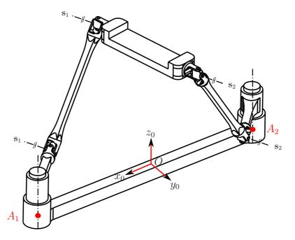
Figure 6: Transition configuration between  $\mathcal{K}_1$  and  $\mathcal{K}_3$ .
