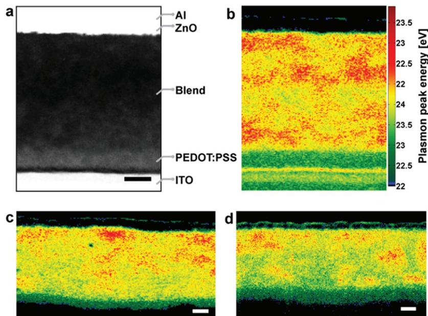
**Figure 5.** a) Annular dark-field image of the lamellar cross-section of the nonannealed device and b) corresponding plasmon peak map using STEM-SI (Scale bars 50 nm). c,d) Plasmon peak maps of cross-sections of devices annealed at 140 °C for c) 1 h and d) 24 h (Scale bars 25 nm); the photoactive layer was processed with DIO.
