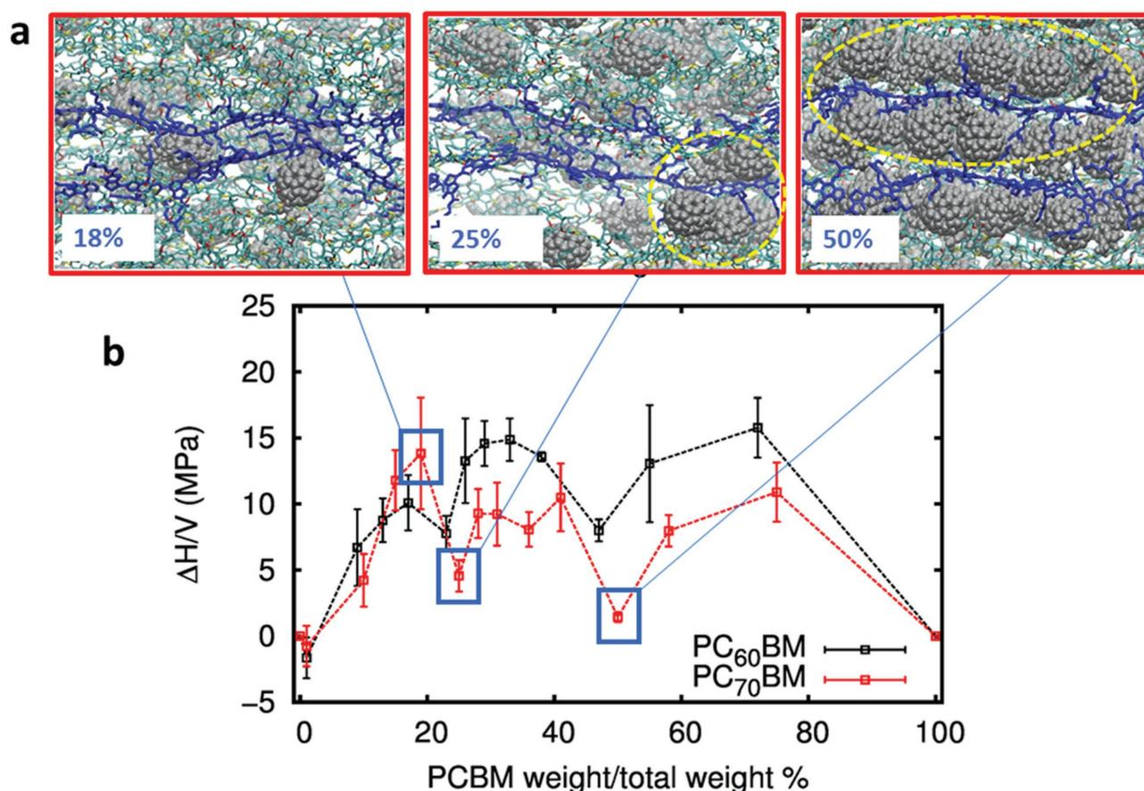
**Figure 3.** a) Calculated PTB7:PC<sub>70</sub>BM blend morphology and b) mixing energy as a function of fullerene (PC<sub>60</sub>BM or PC<sub>70</sub>BM) wt% inside the polymer blend.
