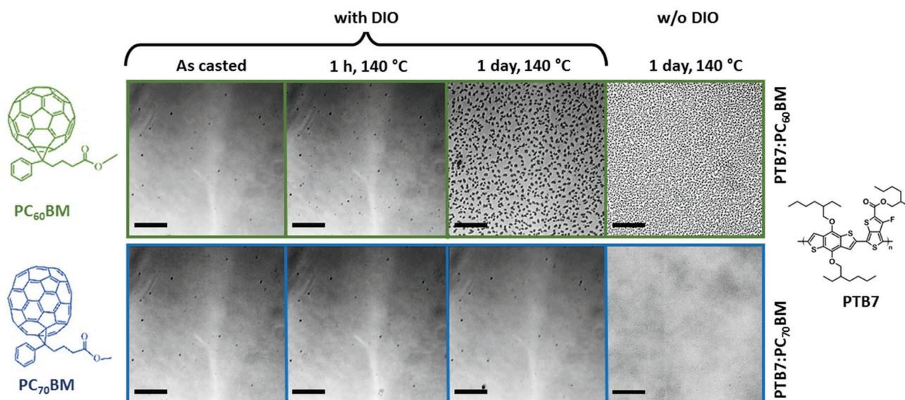
**Figure 1.** Optical images of PTB7:PC<sub>60</sub>BM and PTB7:PC<sub>70</sub>BM blends with and without DIO deposited onto ITO/PEDOT:PSS substrates and exposed to different thermal annealing steps (time, temperature); scale bar correspond to 50  $\mu$ m. Chemical structures of PTB7, PC<sub>60</sub>BM, and PC<sub>70</sub>BM are provided.
