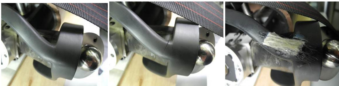
Fig. 6: Clavicle repair. Left : clavicle without loading. Center: Small crack in the clavicle visible under loading. Right: surface repair with fibers and epoxy glue to prevent further damage.
