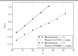
FIG. 2. Exponential divergence of the dynamical susceptibility  $\kappa$ , defined in Eq. (8). We plot  $\log \kappa$  as a function of L, as obtained from the feedback method (points) together with the theoretical prediction (10) (straight lines).
