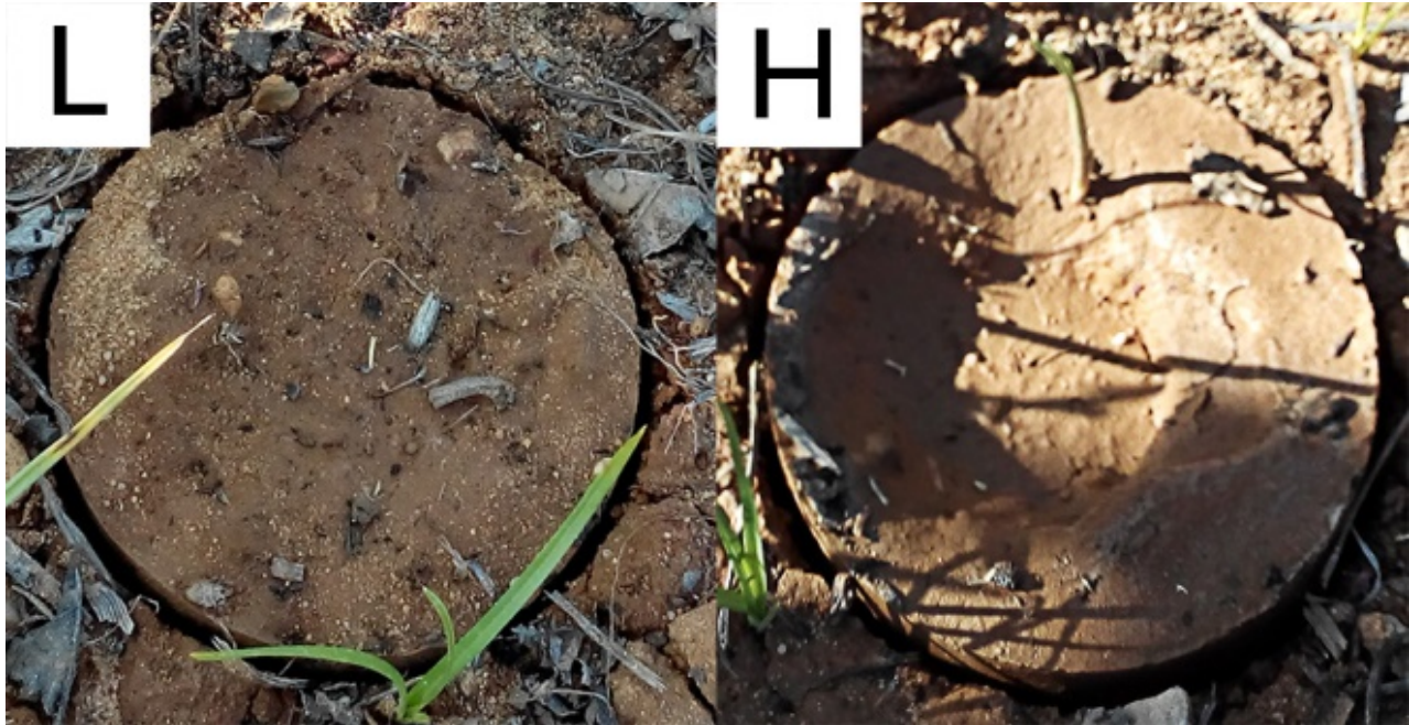
Figure 6. View of the infiltration surfaces after a Beerkan run conducted at low (L) and high (H) height of water pouring.
