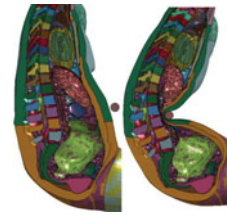
Figure 2. Example of simulation: Hardy et al. (2001) mid-abdomen bar impact at 6 m/s scaled to the subject G14. Another example is provided in Appendix A-3 (see online supplement).
