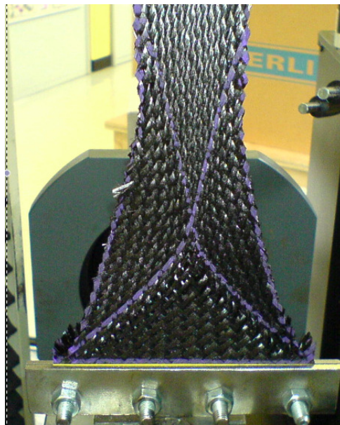
Figure 3: Curvature of the free boundary during the BET
