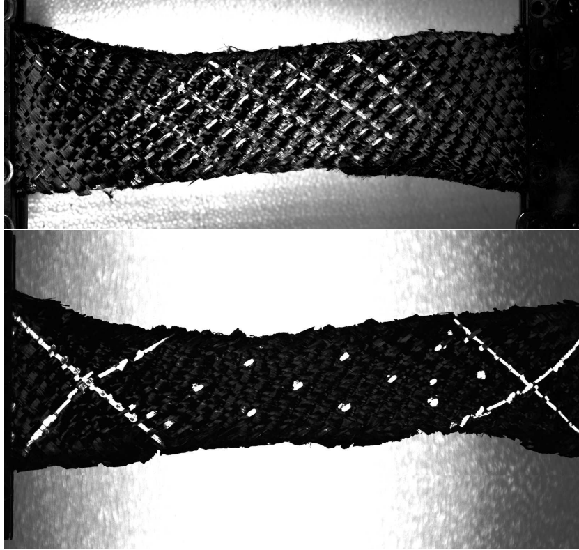
Figure 8: Deformed shape for both specimens (sample I on top, sample II at the bottom)
