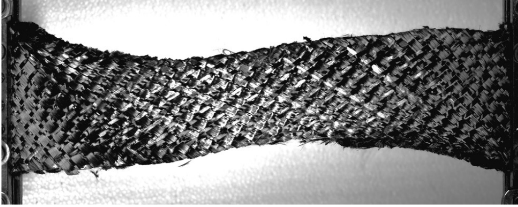
Figure 3: Experimental deformed shape for an imposed displacement u_0 = 56 \text{ mm} .
