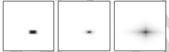
Fig. 5. Examples of shapes for \boldsymbol{\lambda} that can be used with our GRF and SMGRF texture models. The representation is done in the Fourier domain on the reduced frequency domain [-0.5, 0.5] \times [-0.5, 0.5] .
