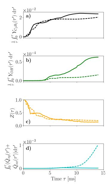
Figure 18. Lagrangian temporal mean mass fraction of  $C_2H_2$ , Lagrangian temporal mean mass fraction of OH, mixture fraction Z, and Lagrangian time integral of the sum of the surface growth and oxidation source terms evolutions for the trajectories of Fig. 17 resulting in a one-peak PSD shape (solid lines) and in a two-peak PSD shape.
