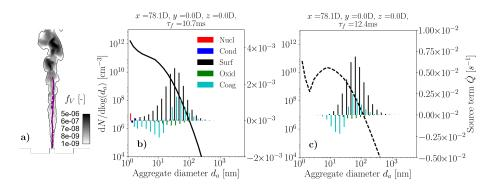
Figure 19. Projected trajectories, in solid purple line for the the trajectory resulting in a onepeak shape and in dashed line for the trajectory resulting in a two-peak shape, are represented with an instantaneous field of soot volume fraction  $f_V$  (a). Final particle size distributions (lines) and final soot sectional source terms (bars) of two Lagrangian trajectories issued from the jet and resulting in a one-peak (b) and two-peak (c) PSD shapes at the same position.
