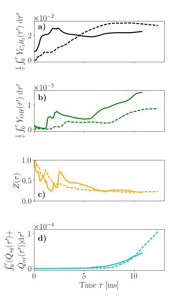
Figure 20. Lagrangian temporal mean mass fraction of  $C_2H_2$ , Lagrangian temporal mean mass fraction of OH, mixture fraction Z, and Lagrangian time integral of the sum of the surface growth and oxidation source terms evolutions for the trajectories of Fig. 19 resulting in a one-peak PSD shape (solid lines) and in a two-peak PSD shape (dashed lines).
