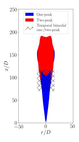
Figure 13. Index of the structure of the particle size distribution (one-peak, two-peak and temporal bimodality).
