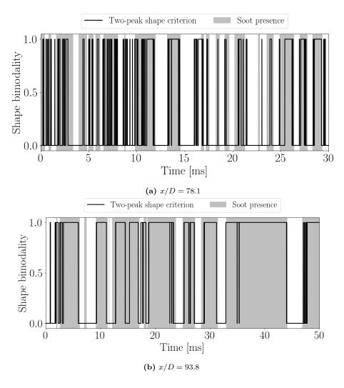
Figure 22. Time evolution of shape bimodality criterion for two selected heights above the burner. A value of 1 corresponds to a two-peak shape, whereas 0 corresponds to a one-peak shape. Soot presence index is indicated in grey filled regions.
