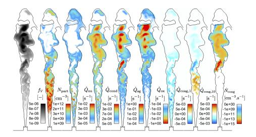
Figure 8. Instantaneous fields of soot volume fraction, particle number density, nucleation, condensation, surface growth and oxidation volume source terms for all the sections, volume coagulation source term for the first and tenth section and number coagulation source term for all the sections. The iso-contour of mixture fraction at  $Z_0$  (indicating the flame front) is shown in solid line.
