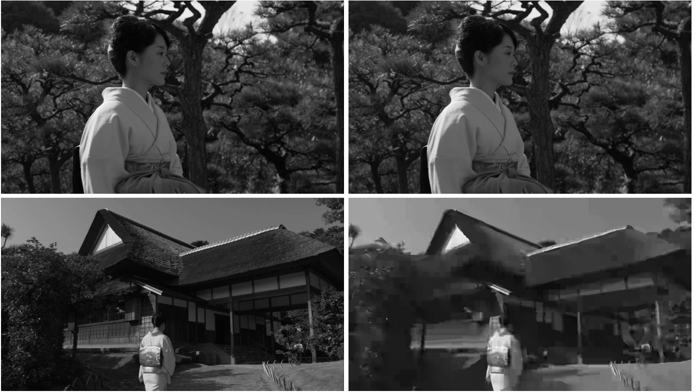
Figure 7. Subjective quality of sequence Kimono at 10 Mbps for two different frames (Left: Proposed, Right: HM R- \lambda )
