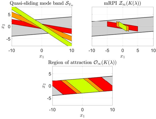
Fig. 2. The set of state constraints  $\mathcal{X}^2$  (grey), the quasi-sliding mode bands (top left), the mRPI (top right) and the region of attraction (bottom) for  $\lambda = 0.2$  (red)  $\lambda = 0.4$  (orange), and  $\lambda = 0.6$  (yellow).
