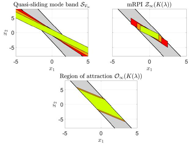
Fig. 1. The set of state constraints  $\mathcal{X}1$  (grey), the quasi-sliding mode bands (top left), the mRPI (top right) and the region of attraction (bottom) for  $\lambda = 0.2$  (red)  $\lambda = 0.4$  (orange), and  $\lambda = 0.6$  (yellow).
