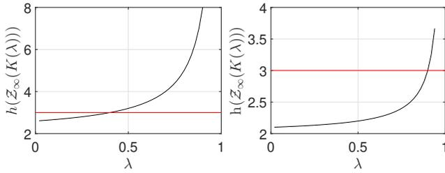
Fig. 3. Relation between  $\|h(\mathcal{Z}_\infty(K(\lambda)))\|_\infty$  and  $\lambda$  for  $\mathcal{X}^1$  (left) and  $\mathcal{X}^2$  (right). The red-line corresponds to  $h(\mathcal{Z}_\infty(K(\lambda))) = \underline{g} = \bar{g} = 3$ .
