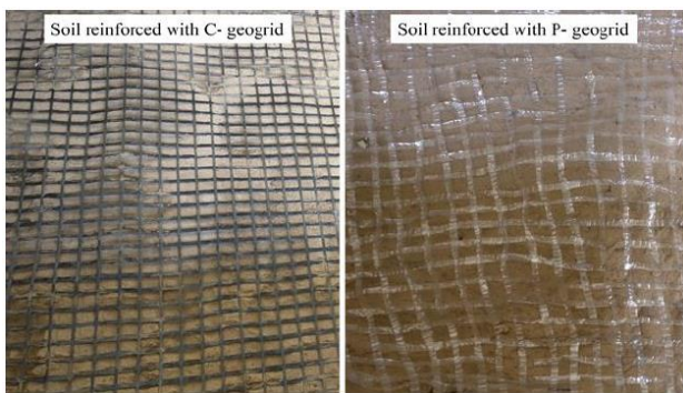
Figure 8. Soil reinforced with conventional geogrid (C) and PET derived geogrid (P) (Dave and Thaker).
