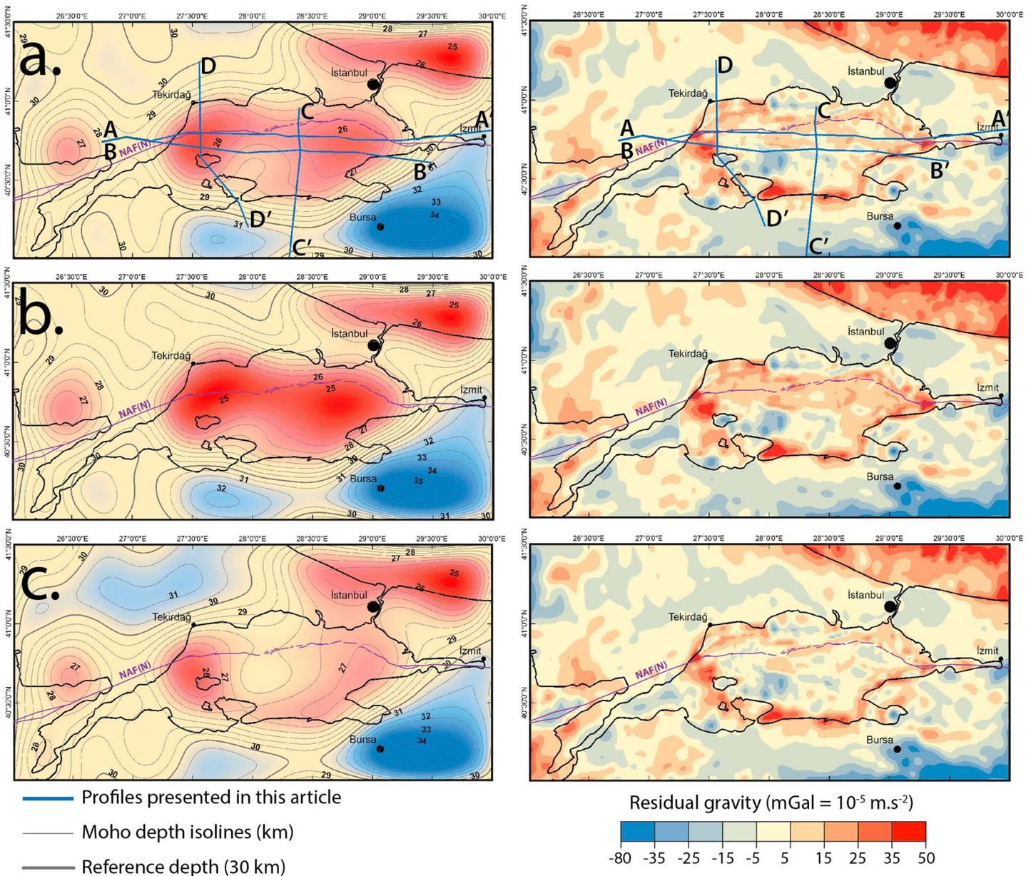
**Figure 6.** Moho depth topography and gravity residual computed with variable density for the synkinematic sediment layer and the prekinematic sediment layer with, respectively, (a) 2.23 and 2.59  $\text{g cm}^{-3}$ , (b) 2.07 and 2.53  $\text{g cm}^{-3}$ , and (c) 2.39 and 2.65  $\text{g cm}^{-3}$ . Thick blue lines: locations of profiles presented in Figure 7.
