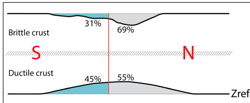
**Figure 11.** Schematic 2-D illustration of the comparison between the basin volume in the upper crust and the Moho uplift in the lower crust. Considering that these volumes are proxies for the stretching and that lower crust thinning that is not proportionally observed in the upper crust implies ductile flow, we find that 14% of the uplift in the lower crust is shifted from the northern block (N) to the southern block (S) and is related to lateral ductile flow.
