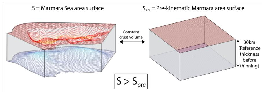
**Figure 10.** Schematic explanation of the extension surface calculation. The surface difference between the current model and the ideal prekinematic model corresponds to the extension. We compute the prekinematic block surface regardless of its shape.
