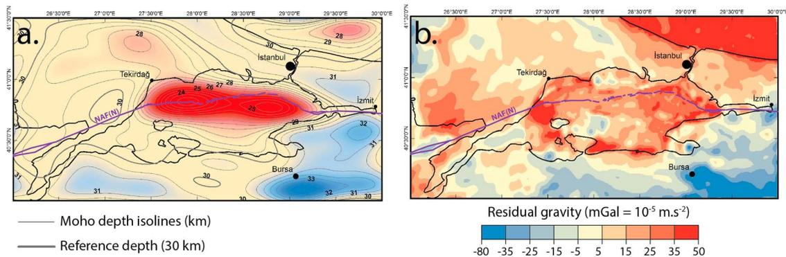
**Figure 8.** (a) Moho depth and (b) gravity residual of the isostatic model. Geological setting, gravity data, and sediment characteristics used as inputs are the same as in the previous models. The compensation depth is 35 km, and the reference crust thickness is 30 km. The Moho topography is filtered to discard small wavelengths. Apart from the filtering, it is a direct response to the geological model.
