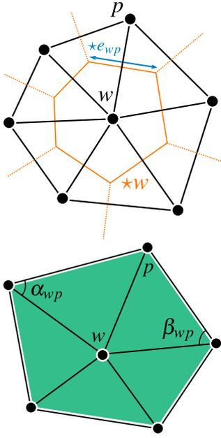
**Fig. 2** Illustration of  $\mathcal{L}_{DEC}$  (top), and  $\mathcal{L}_{COT}$  (down) on triangular meshes. For  $\mathcal{L}_{COT}$  the area of integration  $A_w$  is one third the area of all triangles incident on vertex  $w$  in green. For  $\mathcal{L}_{DEC}$ , we represent the Voronoi dual structure in orange. The dual of the edge  $e_{wp}$  is in blue.
