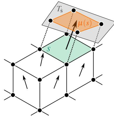
**Fig. 4** Black dots represent the pointels, black segments are the linels. The measure  $\mu(s)$  (in orange) of a surfel  $s$  (in green) is the area of the projection of  $s$  onto the tangent plane induced by the estimated normal.
