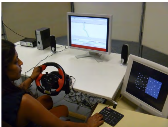
Fig. 2 Experimental set-up for the triple task scenario which combines visual tracking task, SuRT and TDRT
