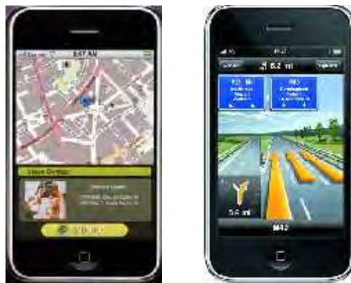
Figure 3: Example of display for ride sharing smartphone application informing the driver about the location on real time of a pedestrian belonging to the community and asking for a ride. This application raises several issues in terms of distracting effect on the driver in addition to personal data privacy.
