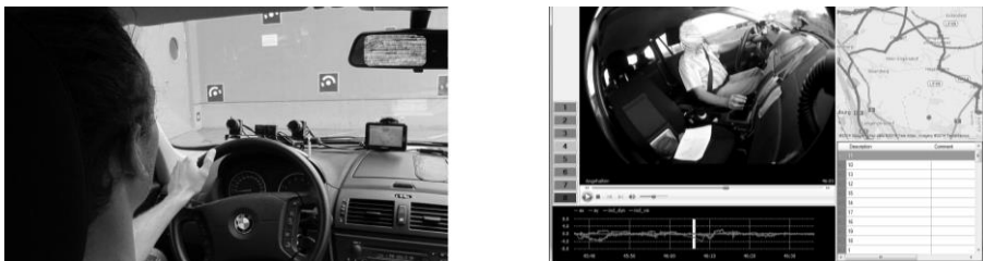
Fig. 1: Eye-tracking and navigation systems in test vehicle (left), data visualisation tool (right). Source: AIT.
