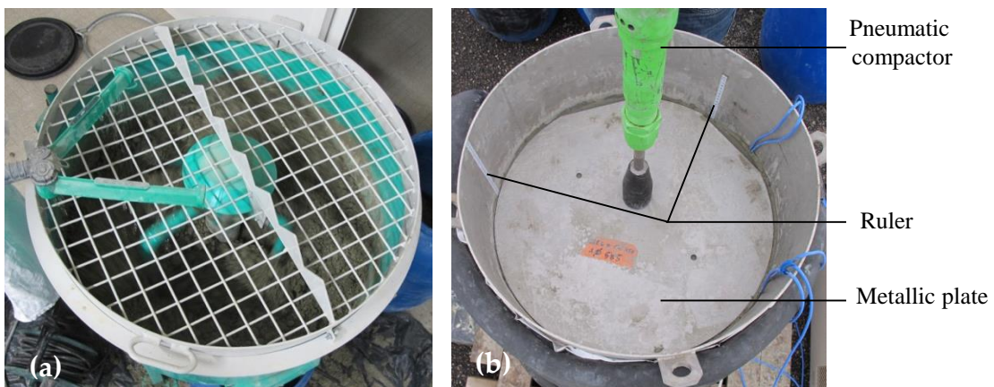
Figure 3. Sample preparation: (a) mixing; (b) compaction.
