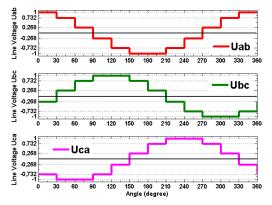
Fig. 12. Three phase six-level output phase-to-phase voltage waveforms
