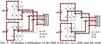
Fig. 5. Switching combination of the fifth cycle  $[\alpha_4, \alpha_5]$  (left) and the sixth cycle  $[\alpha_5, \alpha_6]$  (right)
