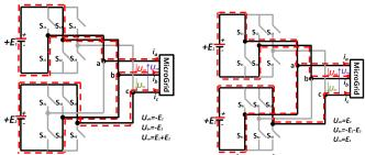
Fig. 7. Switching combination of the ninth cycle  $[\alpha_8, \alpha_9]$  (left) and the tenth cycle  $[\alpha_9, \alpha_{10}]$  (right)
