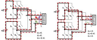
Fig. 4. Switching combination of the third cycle  $[\alpha_2, \alpha_3]$  (left) and the fourth cycle  $[\alpha_3, \alpha_4]$  (right)
