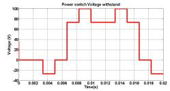
Fig. 15. The voltage across the power switch
