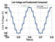
Fig. 14. Inverter phase-to-phase output voltage and its fundamental
