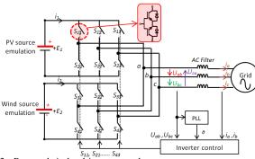
Fig. 2. Proposed six-level inverter topology
