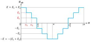
Fig. 9. Six-level output phase-to-phase voltage waveform
