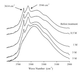
Fig. 6. FTIR spectra of attapulgite before and after treatment with HCl, in  $3800\text{-}2900\,\mathrm{cm^{-1}}$  region.
