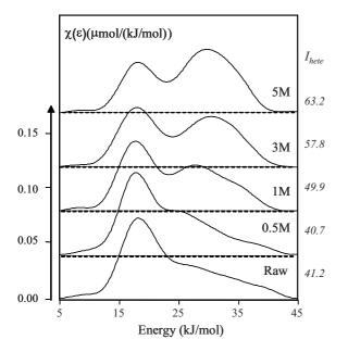
Fig. 11. Adsorption energy distribution functions of the isopropanol probe of the initial and treated attapulgite, measured at 43  $^\circ\text{C}.$
