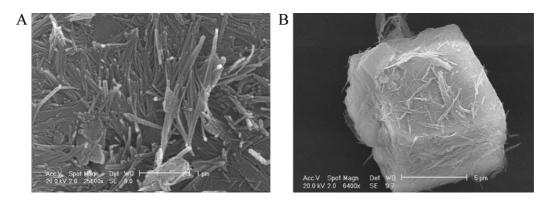
Fig. 2. SEM micrographies of (A) attapulgite fibers and (B) a carbonate inclusion.
