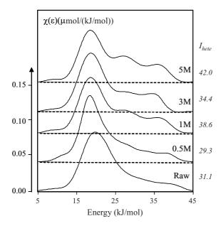
Fig. 12. Adsorption energy distribution functions of the dioxan probe of the initial and treated attapulgite, measured at 51 °C.
