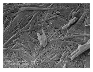
Fig. 4. SEM micrography of attapulgite, after treatment with 5 M HCl.
