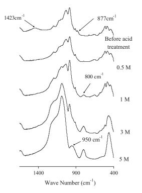
Fig. 7. FTIR spectra of attapulgite before and after treatment with HCl, in the  $1500-400\,{\rm cm}^{-1}$  region.
