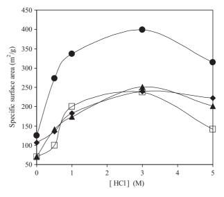
**Fig. 9.** Evolution of the specific surface area of attapulgite treated with various concentrations of HCl, measured by nitrogen adsorption  $\bullet$  and IGC-FC with octane  $\blacklozenge$ , isopropanol  $\Box$ , and dioxan  $\blacktriangle$ .
