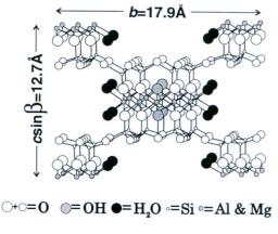
Fig. 1. Crystal structure of attapulgite [21].
