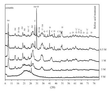
**Fig. 5.** XRD diffractograms of attapulgite before and after acid activation at different HCl concentrations (Att = attapulgite, D = dolomite, C = calcite).
