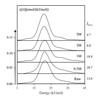
Fig. 10. Adsorption energy distribution functions of the n-octane probe of the initial and treated attapulgite, measured at 53  $^\circ\text{C}.$
