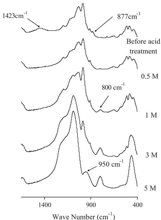
Fig. 7. FTIR spectra of attapulgite before and after treatment with HCl, in the 1500–400  $\text{cm}^{-1}$  region.
