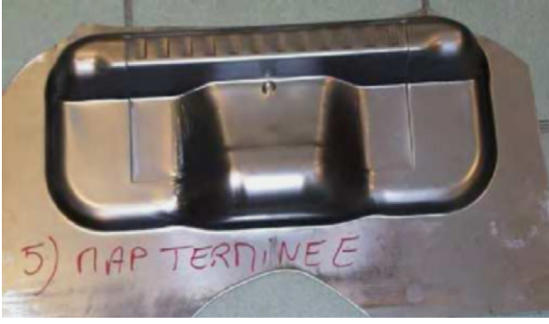
Fig. 4. Stamped part produced by the layered punch. Source: CIRTES.
