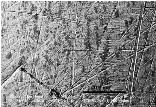
Fig. 16. Die radius degradation for \alpha = 90^\circ , at the entry of the contact (zone E) after 100 cycles.
