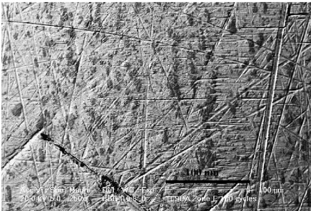
Fig. 16. Die radius degradation for  $\alpha = 90^\circ$ , at the entry of the contact (zone E) after 100 cycles.
