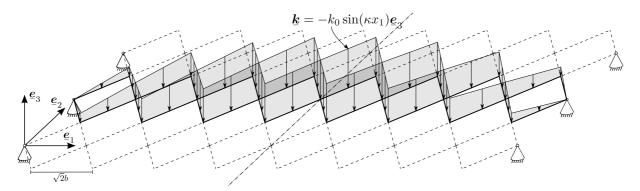
Fig. 3 – Beam lattice configuration at 45° in cylindrical bending configuration
