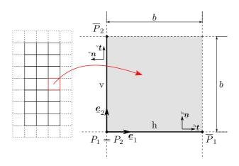
Fig. 2 – The beam lattice unit-cell
