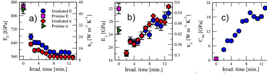
Figure 10: Evolution with irradiation time of (a) the longitudinal and (b) transverse Young's moduli and thermal conductivities as well as of (c) the basal shear elastic constant ( $C_{44}$ ). Values and error bars of  $E_{\parallel}$  and  $\kappa_{\parallel}$  for the IGAR models are based on the average values and deviations, respectively, from simulations performed along  $x$  and  $y$  directions.
