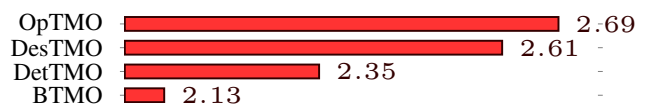
Fig. 16: Computation time in sec (log scale). The time is computed by running all TMOs for an image size (512 × 512) on a Intel Xeon CPU 4 cores processor, 16 Gb RAM windows 7 machine.
