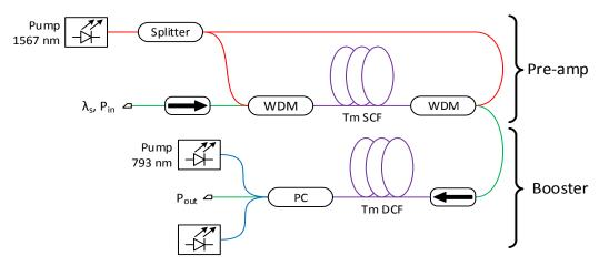
Figure 2: Topology of our two stage hybrid TDFA operating around 2 µm.
