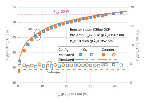
Figure 10: Gain and noise figure versus pump power for the hybrid amplifier based on iXBlue booster in co- and counterpumping.
