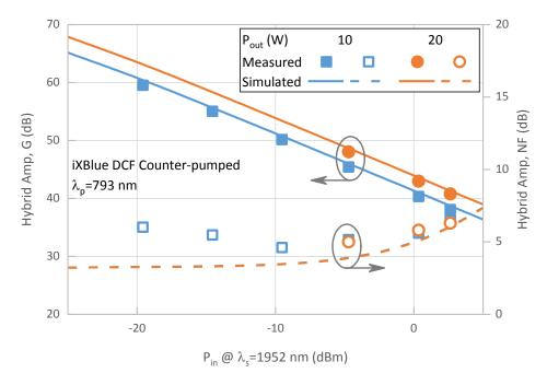
Figure 7: Gain and noise figure versus Pin for the hybrid amplifier based on counter-pumping the iXBlue fiber.
