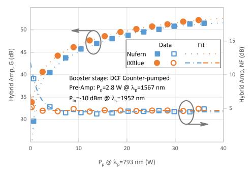
Figure 13: Gain and noise figure versus pump power for the hybrid amplifier with its booster active fiber as iXBlue or Nufern.
