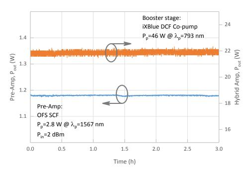
Figure 11: Power stability of the pre-amplifier and the hybrid amplifier at full pump power over three hours.
