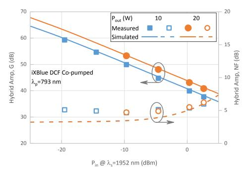
Figure 9: Gain and noise figure versus Pin for the hybrid amplifier based on co-pumping the iXBlue fiber.
