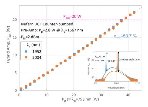
Figure 12: Output power versus pump power for the Nufern hybrid two stage amplifier.
