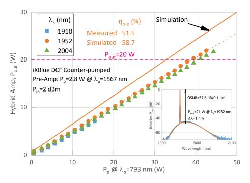
Figure 6: Output power at different wavelengths of the hybrid amplifier versus pump power. Booster stage counter-pumped.
