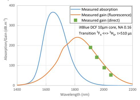
Figure 1: Absorption and gain for the  ${}^{3}F_{4} \Leftrightarrow {}^{3}H_{6}$  transition, measured for iXBlue 10 µm DCF.
