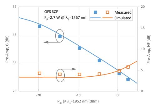
Figure 4: Gain and noise figure of the pre-amplifier versus input signal power at a pump power of 2.7 W.
