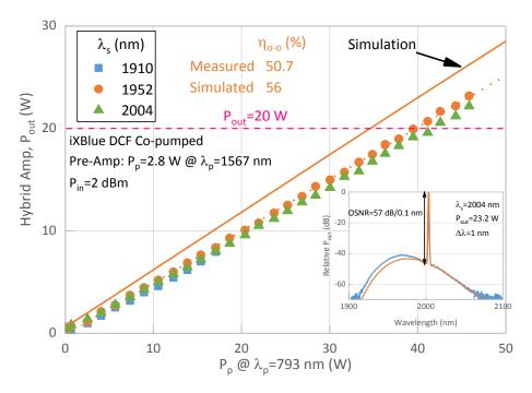
Figure 8: Output power at different wavelengths of the hybrid amplifier versus pump power. Booster stage co-pumped.
