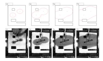
Figure 3: Comparison with infusion experiment
