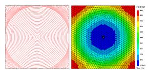
**Figure 2:** Comparison with FEM/VOF (PAM-RTM<sup>TM</sup>)
