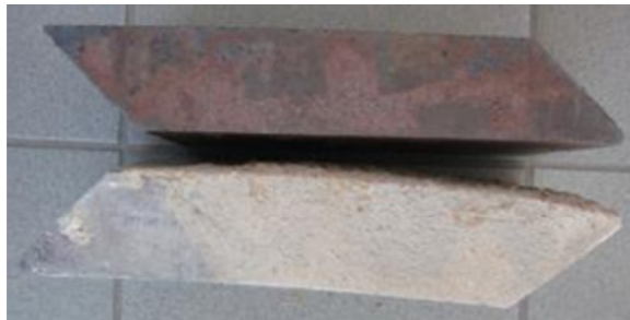
Figure 2: Worn (at the bottom) and new (at the top) tiles.
