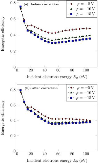
Figure 11:  $R_E(E_0)$  measurement depending on surface charging for silver specimen. These data have been taken before (a) and after (b) EA transfer function correction
