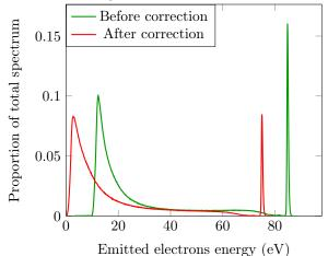
(c) Measured electron energy distribution of silver specimen for  $E_0 = 75 \,\mathrm{eV}$  and  $\varphi = -9 \,\mathrm{V}$
