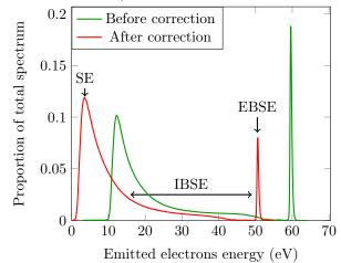
(b) Measured electron energy distribution of silver specimen for  $E_0 = 50 \,\text{eV}$  and  $\varphi = -9 \,\text{V}$
