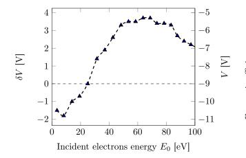
Figure 9: Surface potential V[V] and surface potential variation  $\delta V[V]$  of the SiO<sub>2</sub> specimen as a function of  $E_0$
