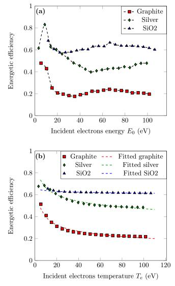
Figure 15: Measurements of  $R_E$  as function of the incident electron energy for mono-energetic incident electron beam of energy  $E_0$  [eV] (a) and for Lambertian distributed incident electron beam of temperature  $T_e$ [eV] (b)
