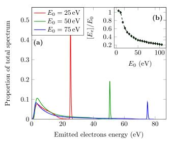
Figure 14: (a) Emitted electrons spectra for three incident electron energy  $E_0$ . (b) : Ratio of emitted electron energy on incident electron energy as a function of incident electrons energy
