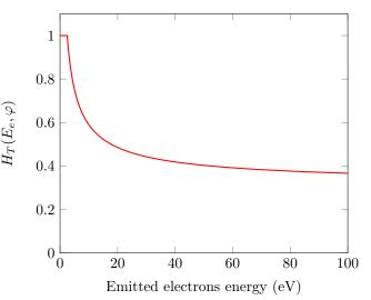
Figure 4: Calculated electron transfer function of transport between the specimen and the electron energy analyzer
