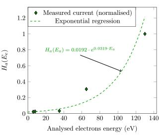
Figure 8: Analyzer EA125 transfer function (normalized), points are experimental data [27], doted line is the exponential regression obtained from equation (13)
