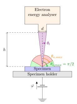
Figure 3: Geometrical scheme of electrons transport between specimen and analyser
