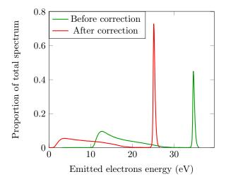
(a) Measured electron energy distribution of silver specimen for  $E_0 = 25 \,\mathrm{eV}$  and  $\varphi = -9 \,\mathrm{V}$
