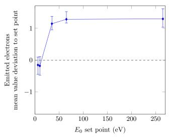
Figure 7: Difference between actual electrons emitted mean energy and set point value
