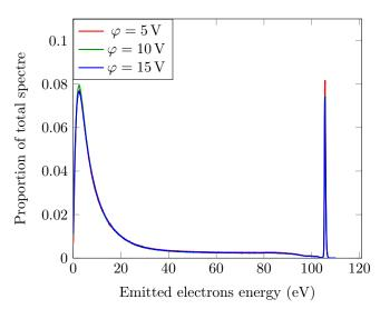
Figure 10: Measured electron energy distribution on silver specimen with  $E_0 = 105 \text{ eV}$  for three biases, in the same experimental conditions as FIG.2, after transfer function correction. Impact of transfer functions correction on spectra measurement
