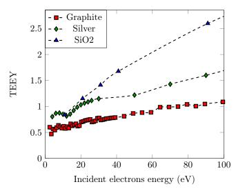
Figure 12: TEEY as a function of the incident electrons energy  $(E_0)$  for three tested materials (SiO2, graphite and silver) [28]
