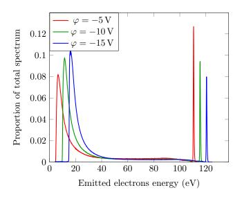
Figure 2: Measured electron energy distribution on silver specimen with  $E_0 = 105 \,\text{eV}$ , for three biases before correction
