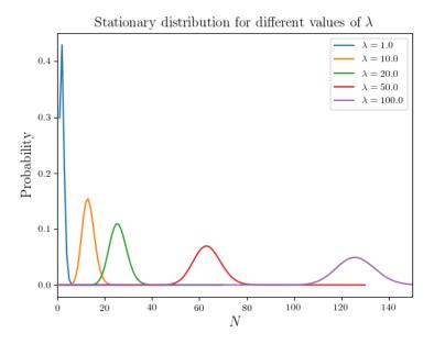
Figure 2: Stationary distribution of the number of tips, for different values of  $\lambda$ . For each value of  $\lambda$ , one can see that the number of tips is really well centered around the average
