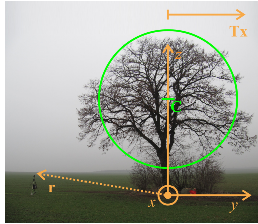
Fig. 8. Single-tree scenario utilized for the experimental validation of the modified PO model and its xyz coordinate system. Rx location is \mathbf{r}=[0, -10, 1.5]\text{m} , and the canopy can be approximated by a sphere of radius 5 m with its center \mathbf{C}=[0, 0, 6]\text{m} . The airship carrying Tx was moving away from the canopy in the y -direction approximately at a height of 200 m above ground level.
