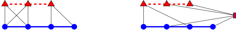
Figure 2: A 1-CIST partition (on the left) and a 1-rooted partition (on the right) of two graphs (circles: V_1 ; triangles: V_2 ; square: A ).
