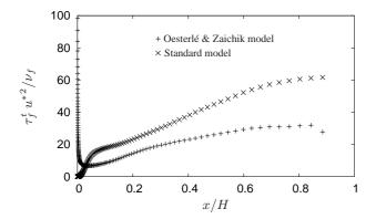
Figure 4: Lagrangian fluid integral time scale predicted by the standard model (+) and by the Oesterlé & Zaichik Model  $(\times)$  [14].
