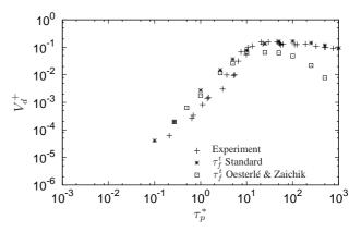
Figure 6: Deposition rate with respect to the Stokes number. Comparison between the experiments of Liu & Agarwal [10], the LBM prediction with  $\tau_f^t$  predicted by the standard model (20) and by the model proposed by Oesterlé & Zaichik (21) [14].
