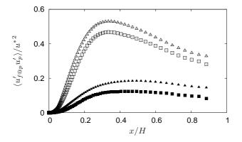
Figure 5: Wall-normal fluid-particle covariance predicted when using the standard model (triangles) and the Oesterlé & Zaichik [14] model (squares). Empty symbols:  $\tau_p^* = 10$  and black-filled symbols  $\tau_p^* = 100$ .
