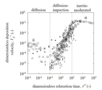
Figure 1: Particle deposition measured in several experiments and gathered by Sippola & Nazaroll [20].
