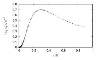
Figure 3: Wall-normal fluid agitation measured by Moser et al. [13] in DNS.
