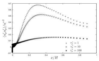
Figure 9: Mean particle variance density predicted by LBM for  $\tau_p^{p} = 1, 10, 100$  with respect to the normalized wall-distance.
